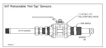
pH measurement on the oxidation towers is often done on the piping between each tower. As mentioned, these applications are less aggressive thus the 547 hot tap sensor or the Barben 546 sensor on a sample line works well. The 546 sensor used 3/4" threads thus can be installed in conventional pipe tees as seen below.
